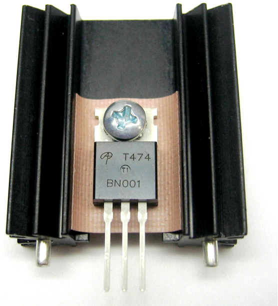
Fig 2: The usable current of small packages is determined by the heatsink they are mounted on
