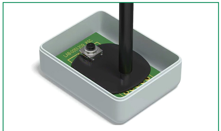
Figure 1: PCB With a KSCXA Tactile Switch. Process of Being Filled With Potting Material
