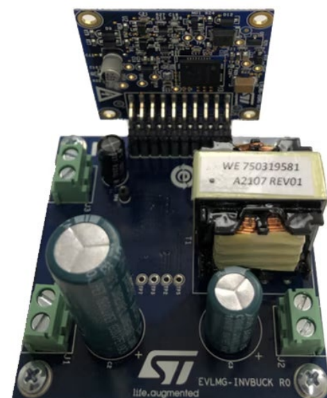
Figure 3: Example of Inverse Buck Demo with MASTERGAN4. (Image source: STMicroelectronics)
