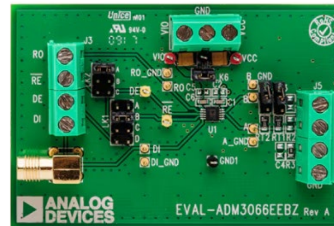
Figure 2: ADI's EVAL-ADM3066EEBZ evaluation board has a footprint for the ADM3066EBRMZ half-duplex RS-485 transceiver in a 10-lead MSOP package. (Image source: Analog Devices, Inc.)
