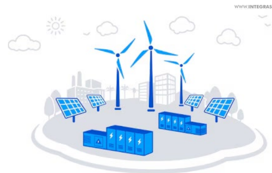
Figure 3: A microgrid can act as a resilient power system for remote areas and communities, such as islands. (Image source: Integra Sources LLC )
